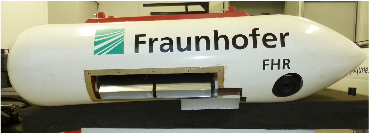
Figure 2-3: Current status of the right wing-pod containing the oblique-looking Ka-band FMCW SAR sensor with slotted wave guides antennas and SAR processing hardware unit. On the right side the integrated PhaseOne VIS camera is visible.
