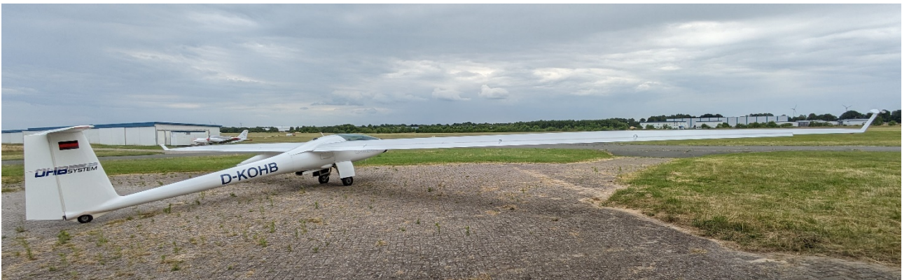
Figure 2-2: IIMEO flight platform used in lieu of a satellite to develop and demonstrate infrastructure monitoring with on-board processing. The image is taken from [5] and shows the plane with only the pod below the left wing attached.
