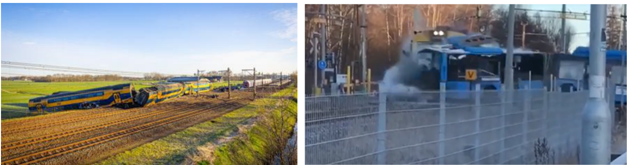
Figure 3-1: Scenes of train accidents caused by different obstacles on the tracks. (left) Maintenance equipment left on the tracks. (right) Stalled bus on the level cross
